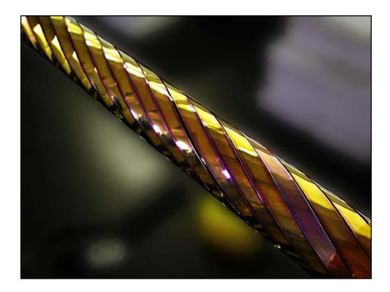
Electric utility companies are presently researching electrical transmission lines constructed of sophisticated high-temperature superconducting cable that delivers more power with greater voltage control and current density. By "high temperature" we mean superconductivity at the temperature of liquid nitrogen. Under normal atmospheric pressure the boiling point of liquid air is approximately 78 K (-319°F) and that of liquid nitrogen approximately 77.2 K (-320.44°F).
