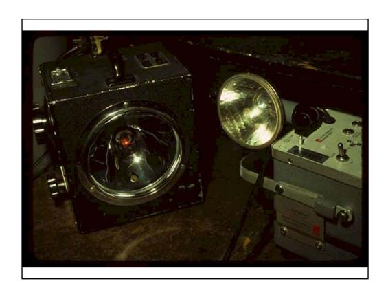
The Edgerton stroboscope is widely used for stop-motion photography and other purposes.
