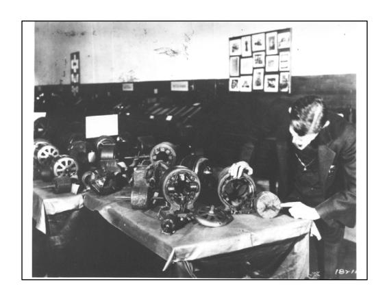
Here is Tesla with an array of poly-phase AC induction motors that embody his rotating magnetic field concept.
