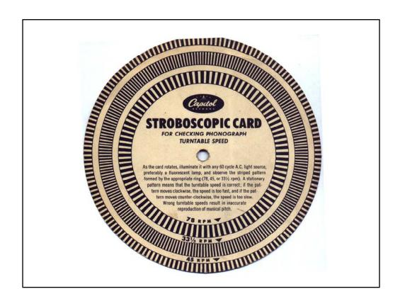
The Stroboscopic Card is for calibrating the speed of rotation of record turntables in order to assure accurate reproduction of musical pitch.
